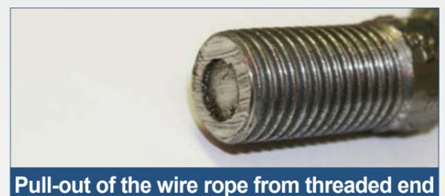
Pull-out of the wire rope from threaded end
