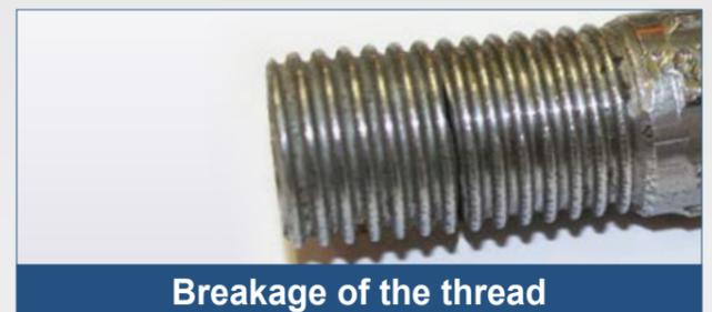
Breakage of the thread
