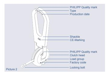
All lifters are designated with the CE symbol according to the machinery directive (2006/42/EG).
