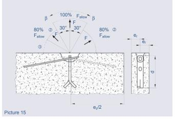
The diagonal tension reinforcement has to be positioned close to the recess former.
