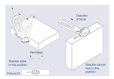
In the upper position, the shackle may lock within the clutch housing. A narrow lifting cable angle will cause the shackle to become bent. The problem can be overcome by turning the shackle through approx. 45° (lower drawing).
