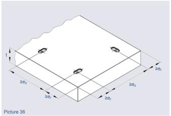
Where loads are acting towards the edge of the element, insert angled pull reinforcement as for spread or two hole anchors.
