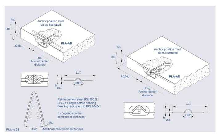
The horizontal legs of the tilting and turning reinforcement are located directly within the outermost position of the reinforced area. Tilting reinforcement on both sides also acts as angled pull reinforcement. No additional angled pull reinforcement is required.
