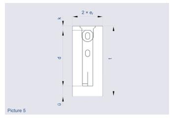
Minimum unit thickness for precast units
