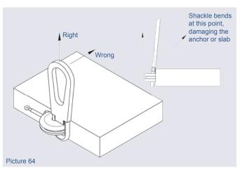
If the shackle is pulled towards the top surface of the slab when subjected to the load, it may become bent on the edge of the slab.
