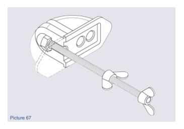
The bayonet holding screw PLA-AK-S2 consists of a threaded holding screw with a pressed-on bayonet fitting. This is inserted into the bayonet connection of the recessed unit and then turned through 90°. The upper wing nut must then be at right-angles to the lengthwise direction of the recessed unit. The recessed former is then drawn onto the formwork with the second wing nut.
