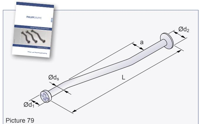
**Table 17: Spherical head anchor - with offset**
