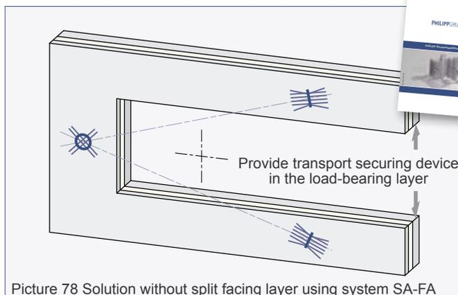
Picture 78 Solution without split facing layer using system SA-FA
