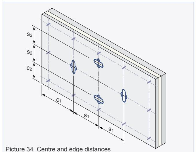
**Table 7: Minimum centre and edge distances of the load-bearing anchors**
