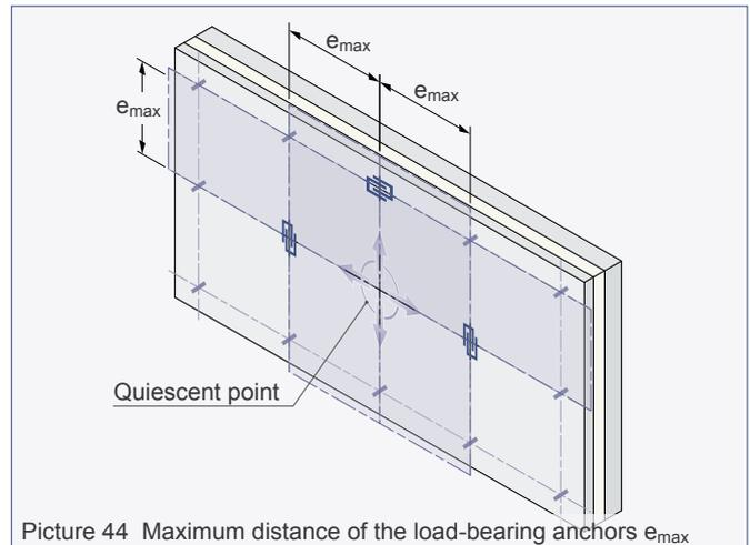
Picture 44 Maximum distance of the load-bearing anchors  $e_{max}$
