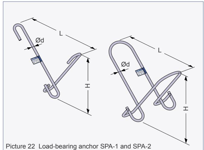
Picture 22 Load-bearing anchor SPA-1 and SPA-2
