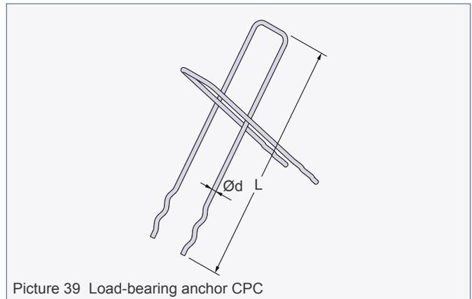
Picture 39 Load-bearing anchor CPC
