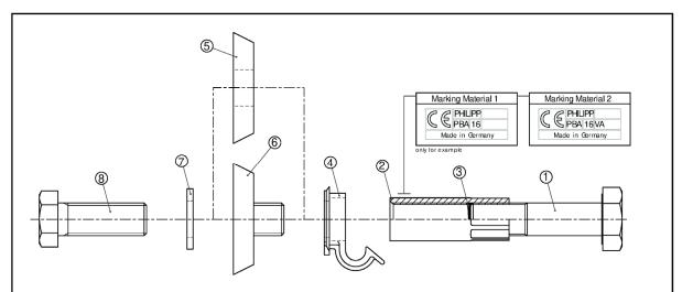
Table A3: Specification and material of the anchor and appropriate components
