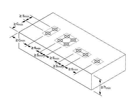
Spacing, edge distance and minimum thickness of concrete member apply also for anchors in front-side installation.
