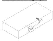
Maximum setting torques max. Tinst for PB Anchor
